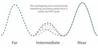
Fig. 2: Schematic drawing showing the utilization of constructive interferences for creating an intermediate peak through EPS technology
