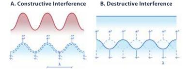
Fig. 1: Schematic illustration of interference patterns: a) Constructive interference - crest of one wave overlaps crest of another wave – reinforcing each other b) Destructive interference - crest of one wave overlaps trough of another wave – cancelling of each other
