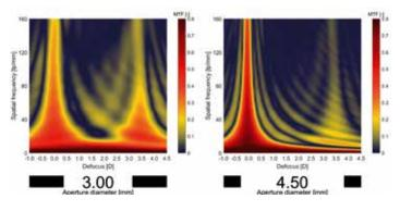
Fig. 5: Pictures of a 3D modulation transfer function (MTF) show light intensity allocation at different aperture sizes. Dark red = strong light intensity. At 3 mm aperture we see excellent performance for near vision with sufficient intensity at intermediate range; at 4.5mm there is strong light intensity for far vision.
